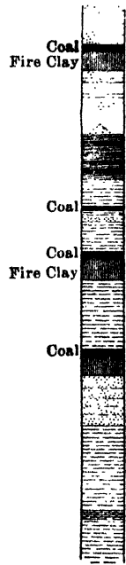
Fig. 2. — Section on coal measures of western Pennsylvania, showing fire clay under coal beds (After Hopkins.)
